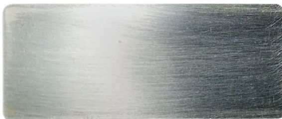
No corrosion as protected by acid scavenger
