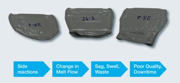
Degraded PCR can cause melt flow issues, like sag, swell, or uneven distribution. BAEROPOL T-Blend 1111 TX keeps your process running with high quality and consistency.
