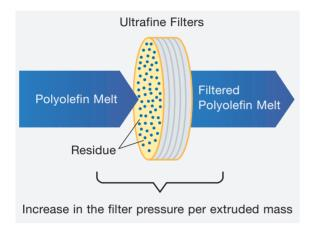
Ceasit FI, designed with high purity and low filtration index, is especially suited for use as acid scavenger/lubricant in polyethylene and polypropylene film and fibre applications where very fine extruder screen packs are used.
