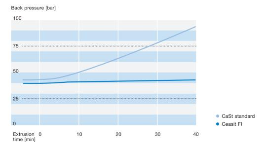
Ceasit FI provides minimal pressure built up over time.
